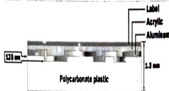
Cross-section of a CD
